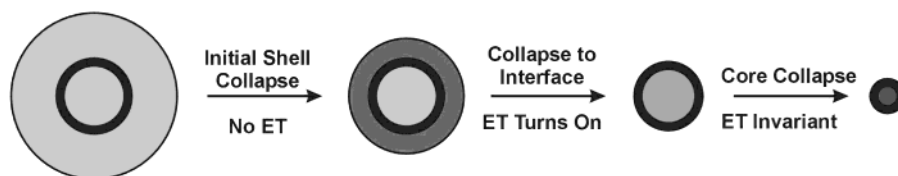
Scheme 1. Proposed Mechanism of Core–Shell Microgel Deswelling
